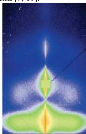
\mu\text{GISAXS} pattern of a self-assembled nanometer-sized gold cluster layer on top of thin polymer layer on a silicon substrate [10].
